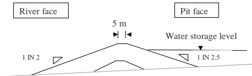
Figure 3: Curragh North mine site flood levee typical cross section
